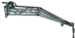
自升降起吊弯臂 Angle crane jib with winch
